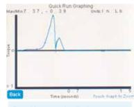
Resulting graph displays torque vs. time. Tap an area of the graph to zoom up to 4 times the size.
