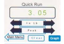
Use Quick Run mode to perform a single run torque test and view a graph of the results.
